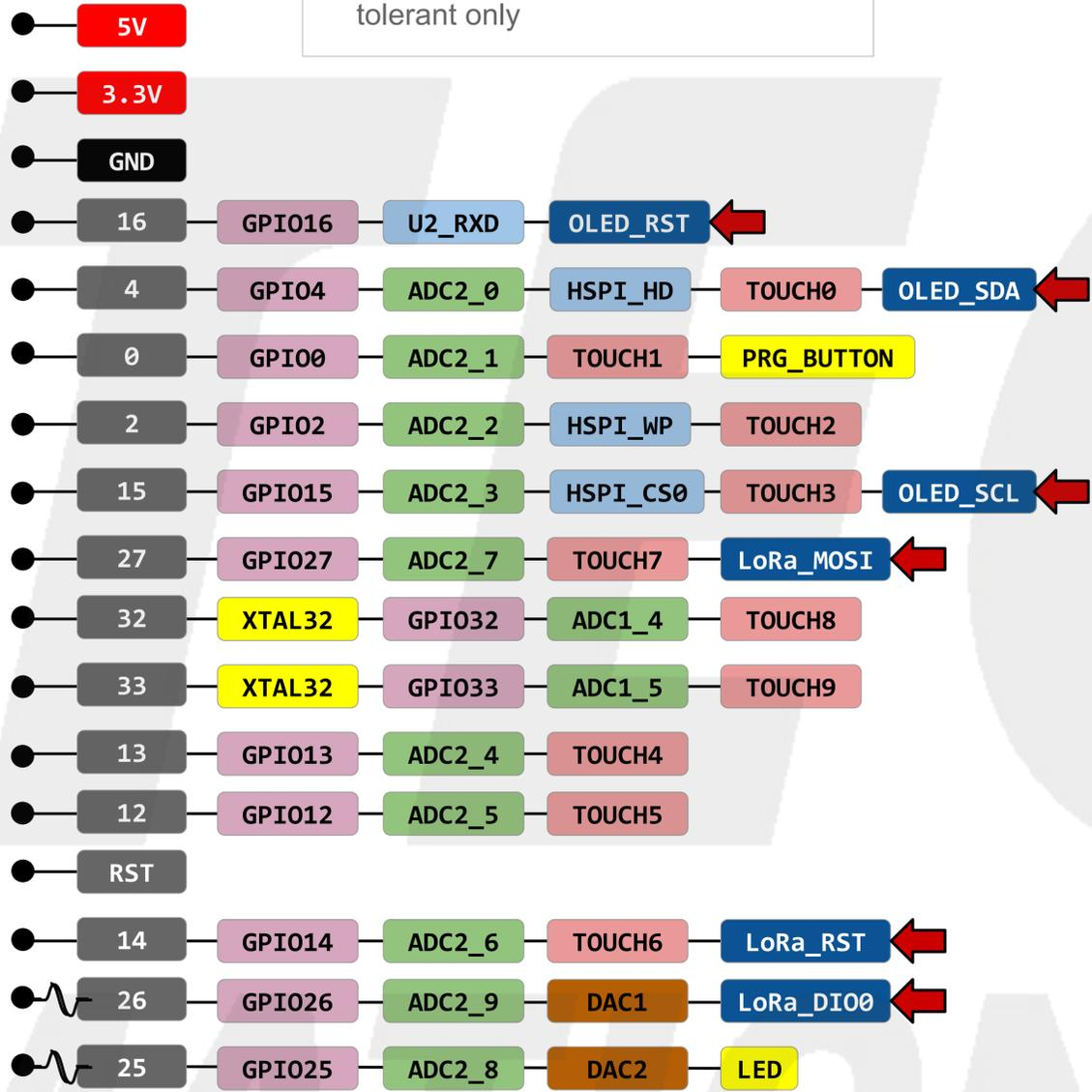
Pins with this arrow are used by on-board OLED or LoRa, they must not be used for other purpose unless you know what you are doing!
