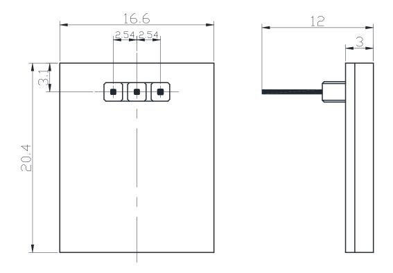
Figure 3-4 HTTM-SC Single key module size
