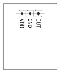
figure 3-2 Pin definition of single-key module
