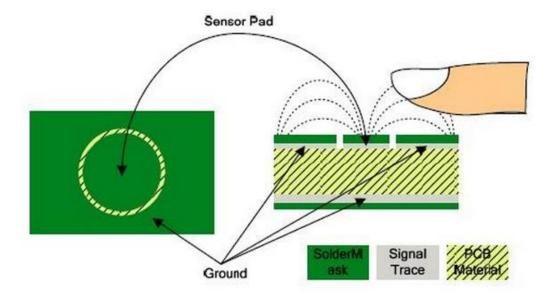
figure 3-1 Principle sketch of touch key
