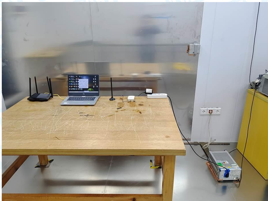
Photo of Setup for Conducted Emission
