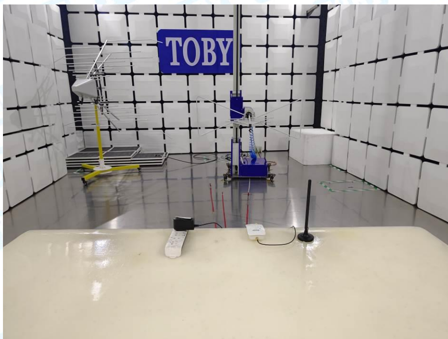
Photo of Setup for Conducted Emission
