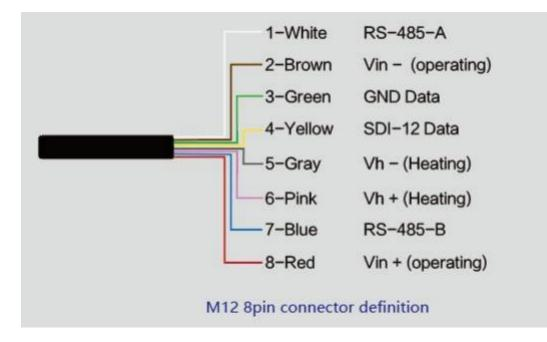
The device adopts an M12 8-pin connector, the different colored pins provide power and data communication (as shown in the above diagram).
