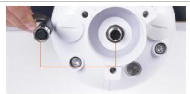
Plugin the cable and tighten it clockwise
