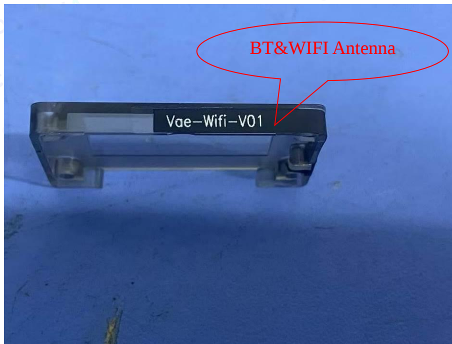
Photo 12 Internal of Antenna
